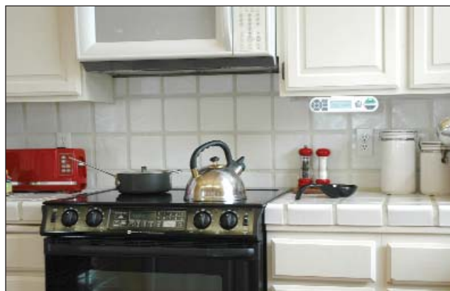
The built-in motion detector in CookStop “knows” if the resident leaves the kitchen and automatically shuts off the stove or cook-top (John Knox Village).
